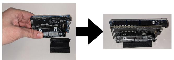
**Step 3)** Plug in micro USB cable at the board side. Leave Type A side unplugged until later.
